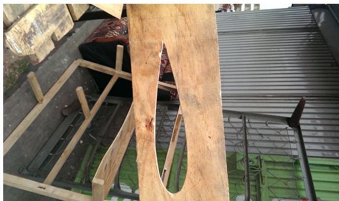
Fig. 2. Cut out NACA 0021 airfoil profile
