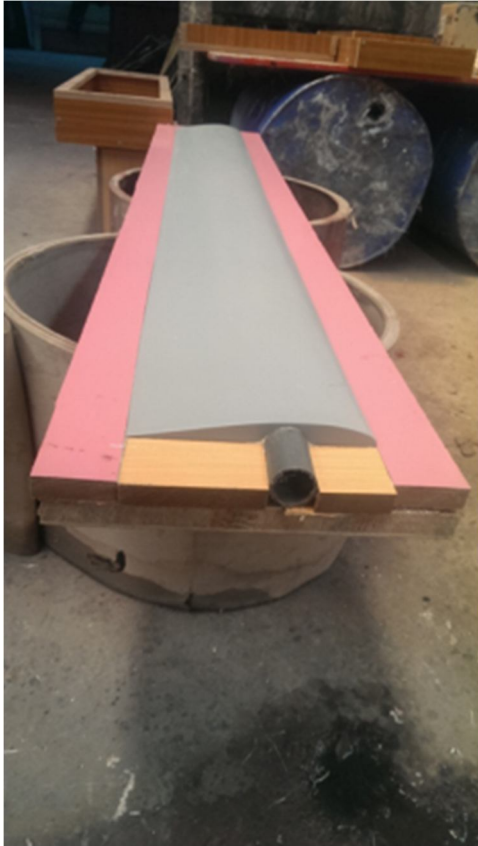
Fig. 4. The wooden blade master copy was used to make the GFRP mould
