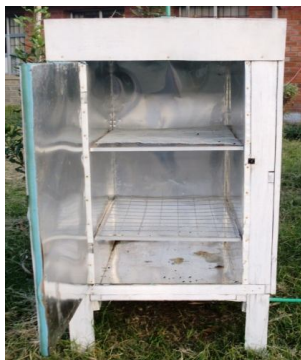
Fig. 3. An unloaded near infrared reflecting (NIR) charcoal cooler
