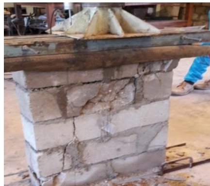
Plate 4.1: Failure patterns of silicate limestone wall
