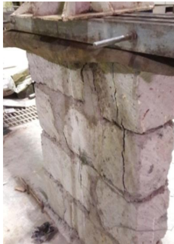
Plate 4.3: Failure patterns of natural stone wall
