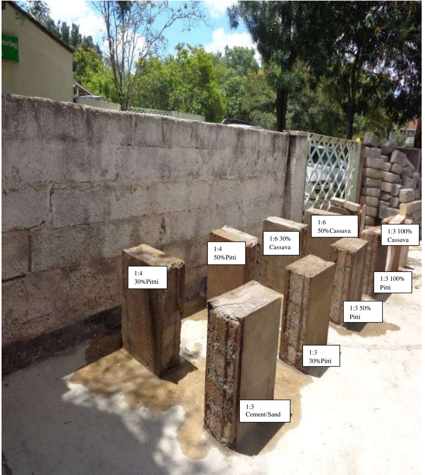
Plate 3.4: The walls plastered with different mortar mix
