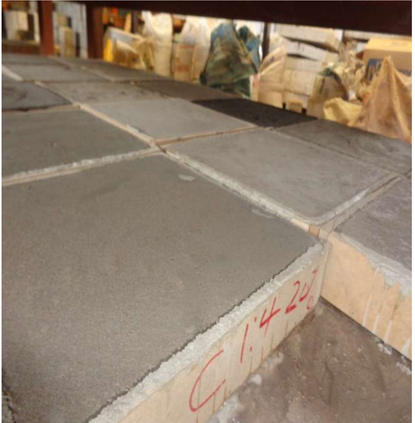
Plate 5: Showing different specimens cast for shrinkage test
