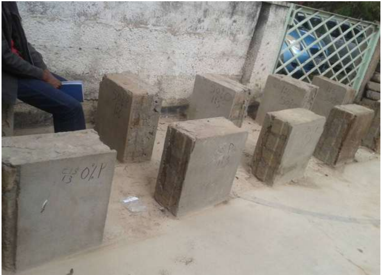
Plate 4: Showing walls plastered with different mortar mix
