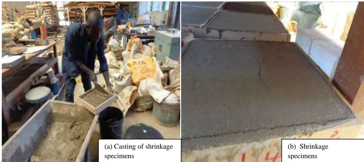
Plate 3.1: The casting of the shrinkage specimens
