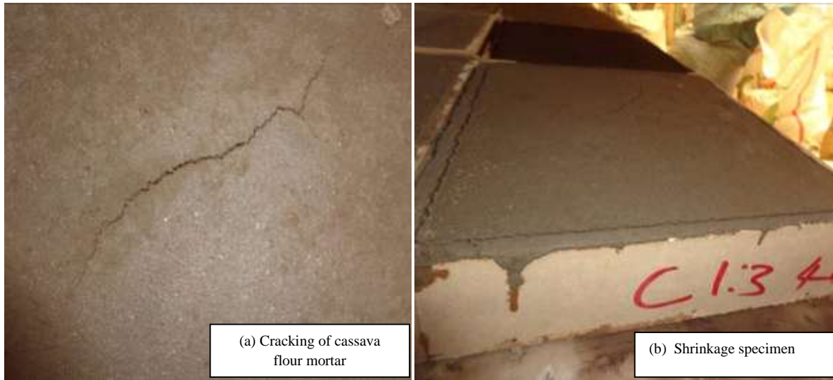
Plate 4.1: The cracking of cassava flour mortar
