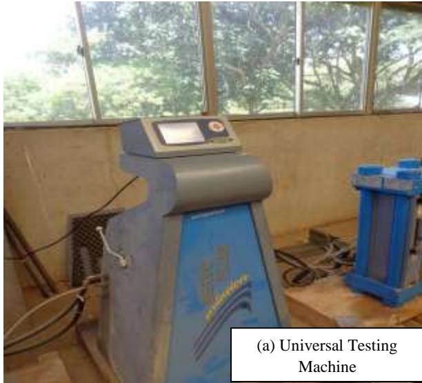
Plate 3.2: The Universal Testing Machine and cast cubes
