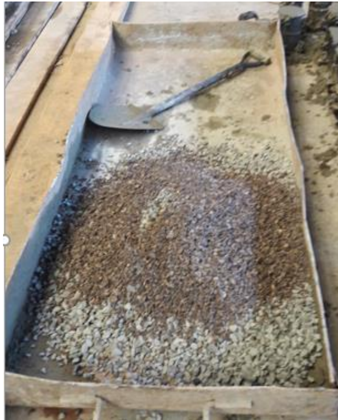
Figure 3-2: Tray used for the mixing of concrete
