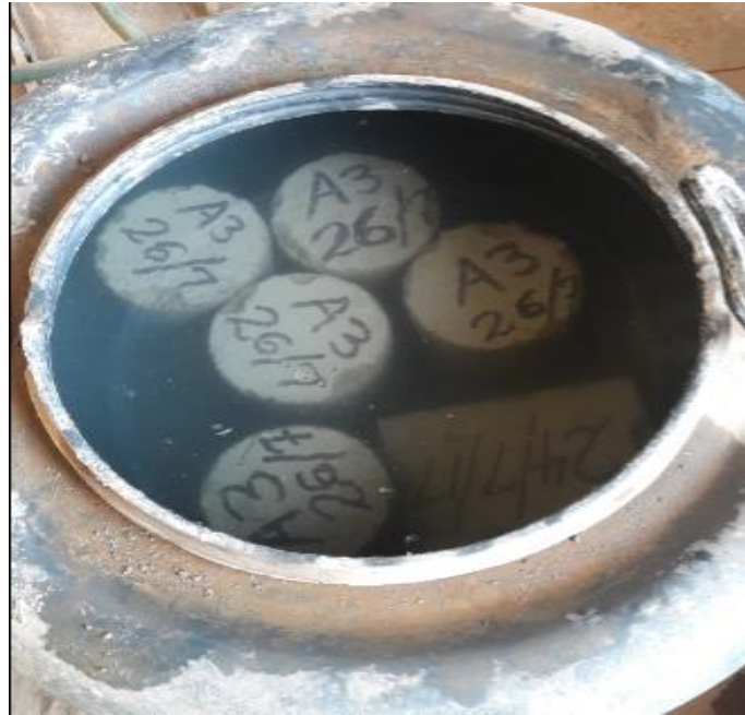
Figure 3-3: Curing of concrete by immersion
