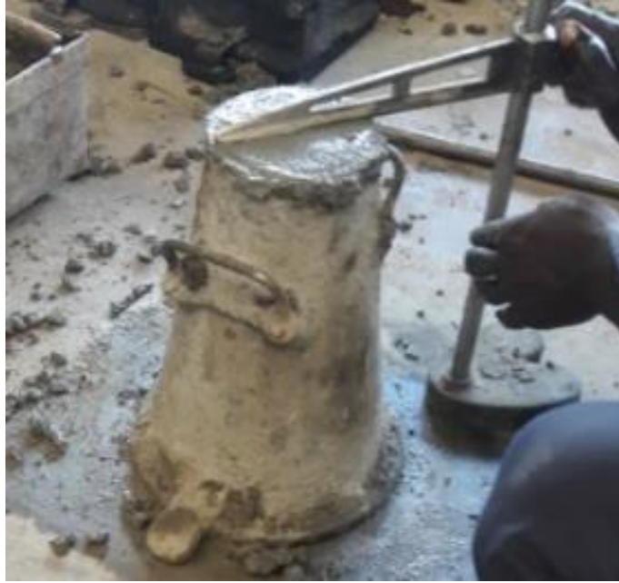
Figure 3-4: Determination of slump as per BS 1881-102 (1983)
