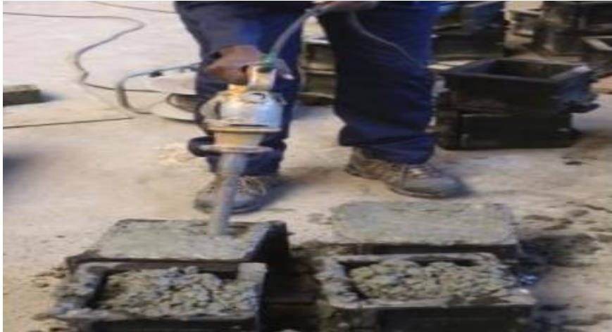
Figure 3.5: Casting and compacting concrete into the concrete molds
