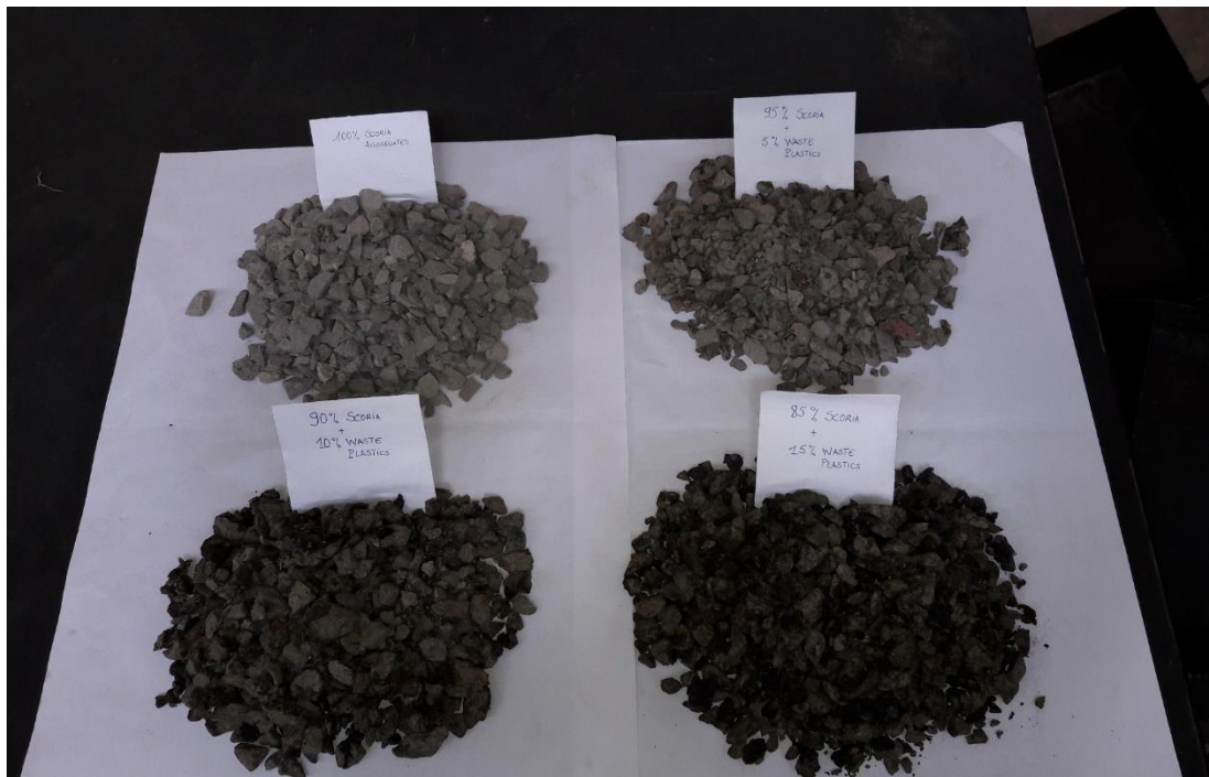
Plate 3.2: Pre-coated volcanic scoria aggregates at different percentages of waste plastics on scoria aggregates (0%, 5%, 10%, and 15%)
