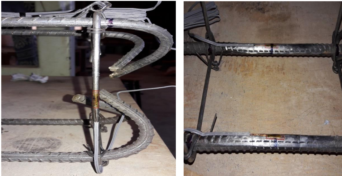
Plates 3.13: Strain gauges mounted on reinforcements.
