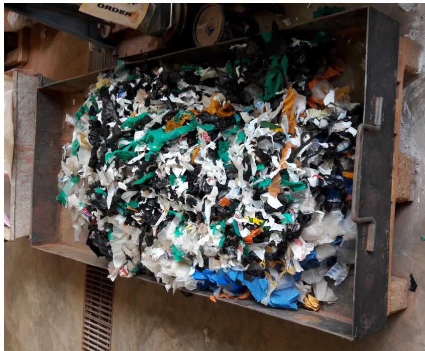
Plate 3.5: waste plastics washed and shredded
