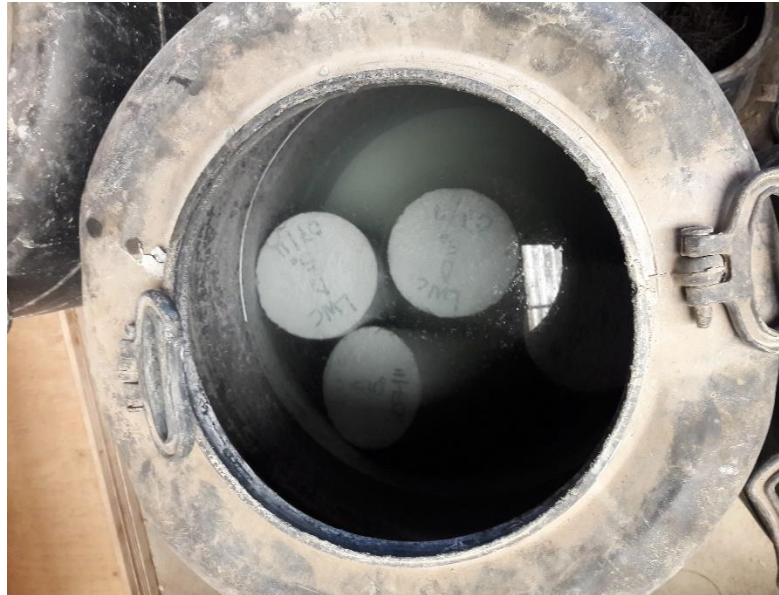
. Plates 3.8: Curing process of cylinders and cubes in tanks.
