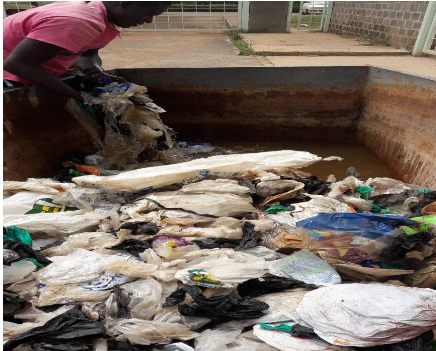
Plate 3.4: washing process of waste plastics
