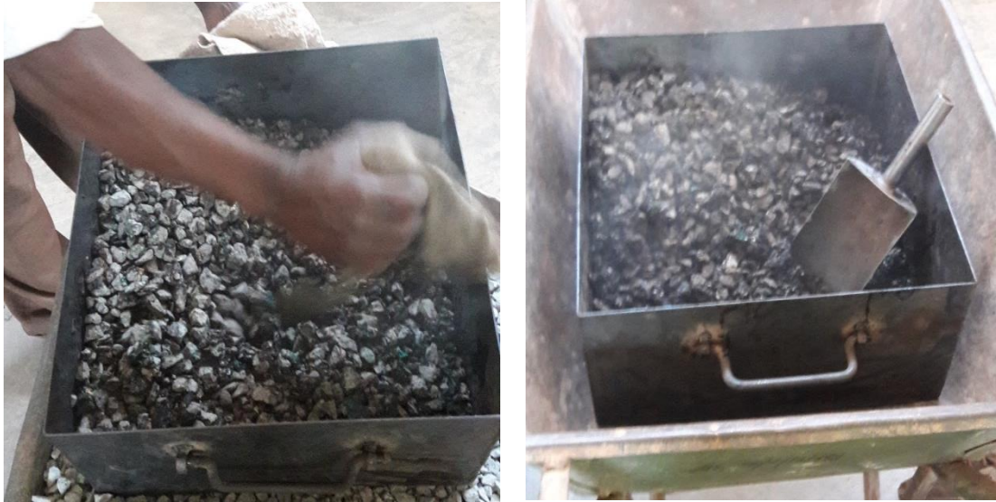
Plate 3.6: Pre-coating process of volcanic scoria aggregates with waste plastics (mixing).
