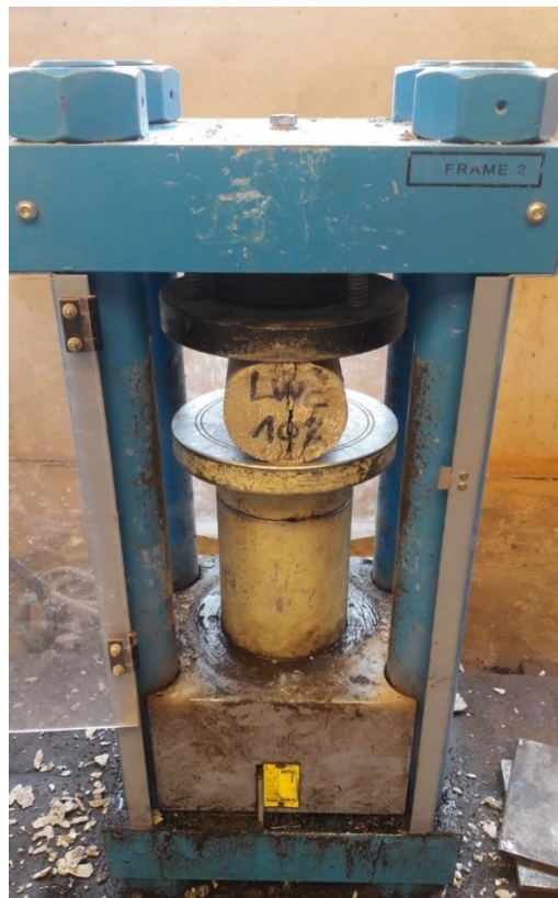
Plate 3.11: Splitting tensile test
