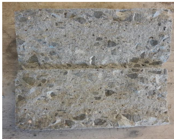
Plate 4.1: Cylinder specimen split at the required age to evaluate the chloride penetration depth.
