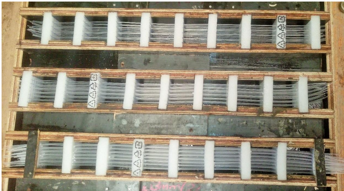
Figure 3.15 Cubic molds for compressive strength and light transmittance tests
