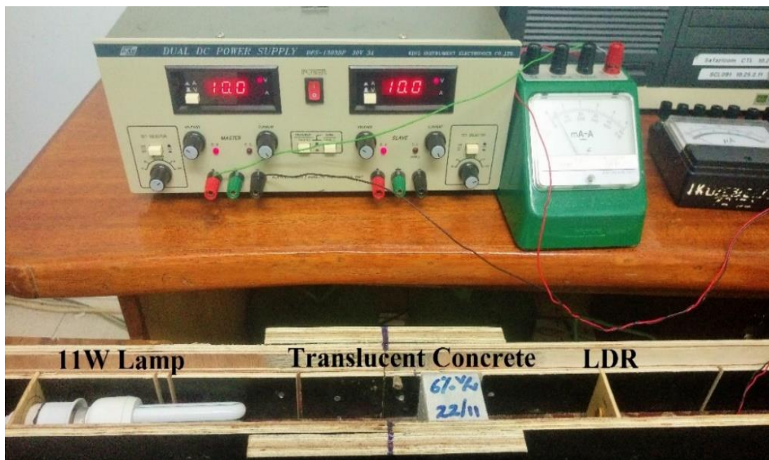
Figure 3.21 Experimental setup and arrangement of light transmittance test
