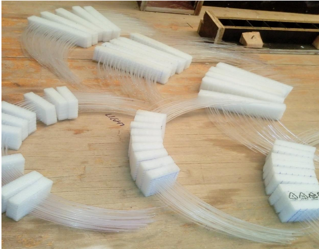
Figure 3.14 Fixing and inserting of plastic optical fibers through low-density polyethylene (LDPE) sheets
