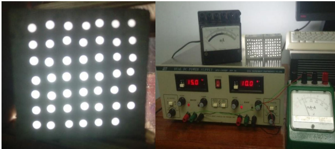
(a) Typical translucent concrete (Ø2mm, 6% POF)
