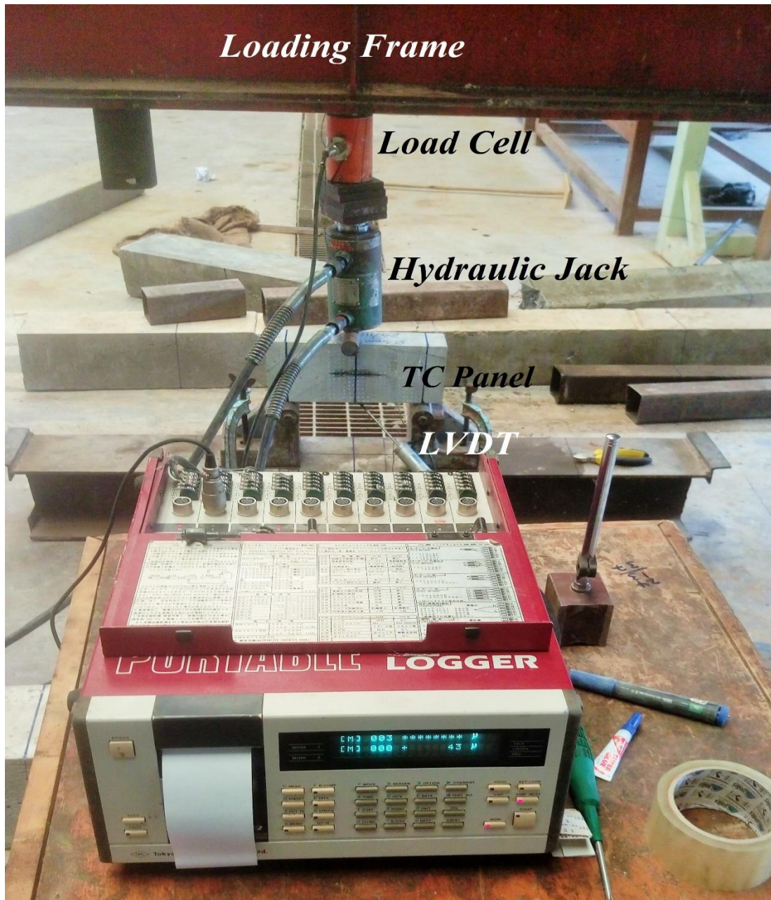
Figure 3.27 Experimental test setup arrangement of structural performance of translucent concrete panel
