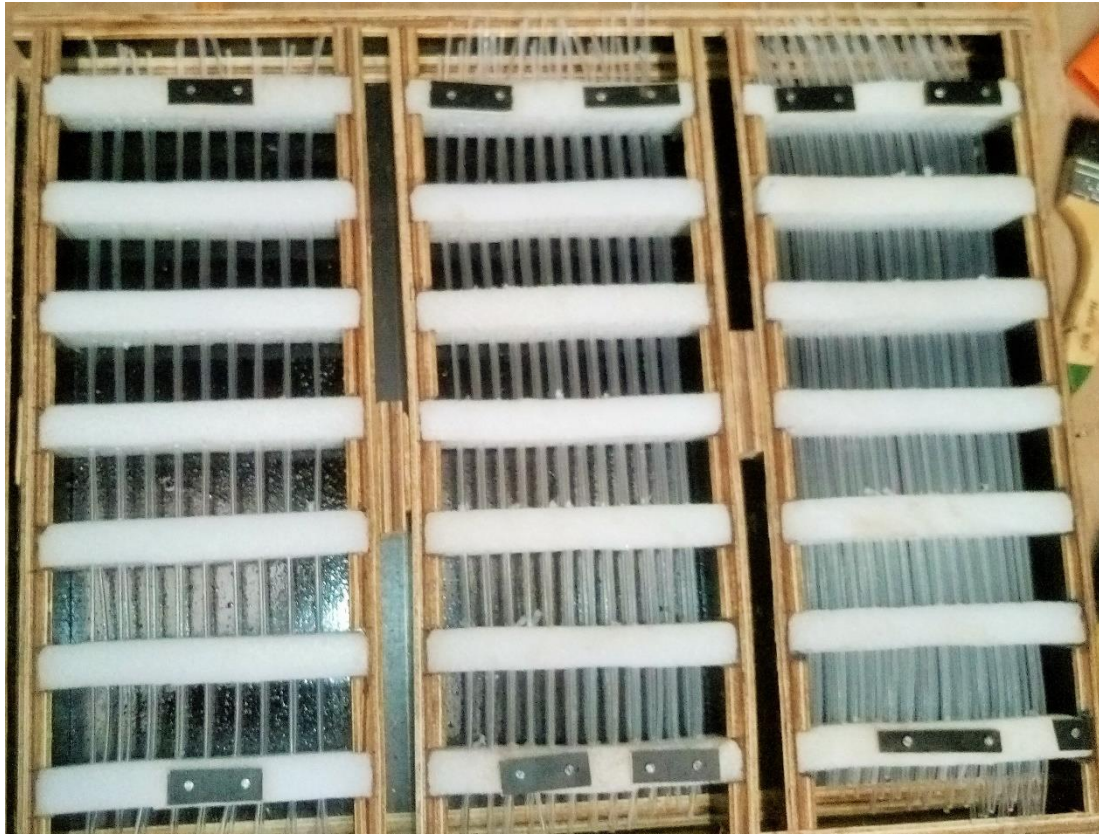
Figure 3.16 Prism molds for the flexural strength test
