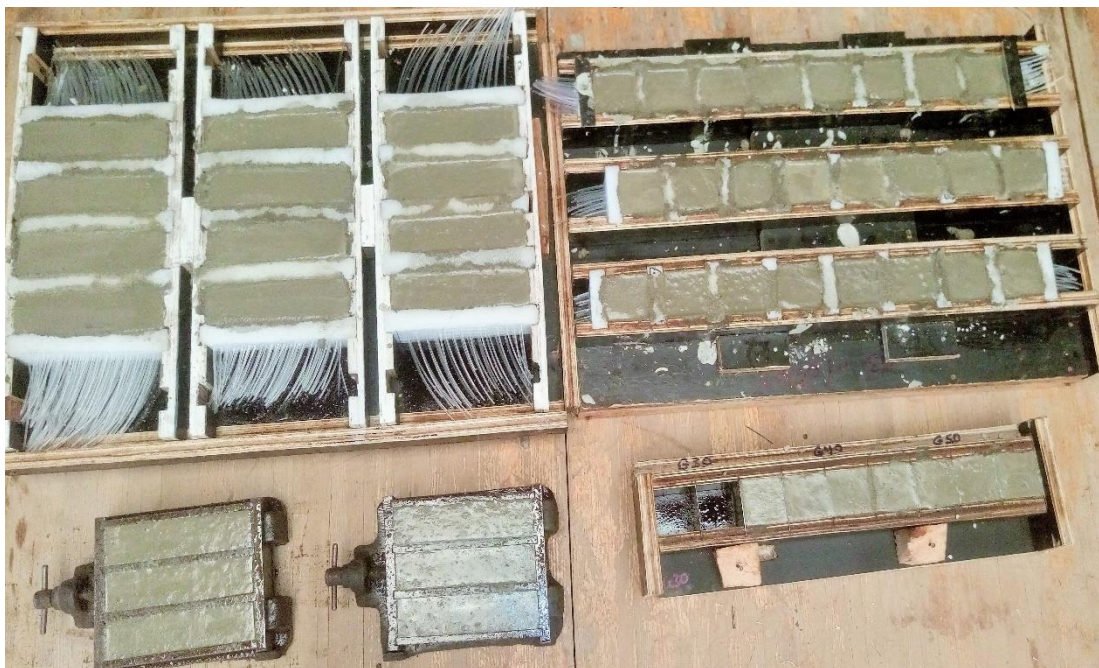
Figure 3.17 Concrete casting of translucent concrete specimens
