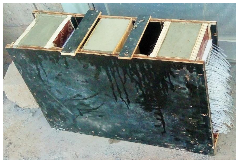
Figure 3.24 Pre-cast translucent concrete panel specimens
