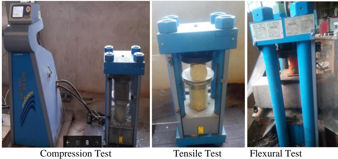
Figure 3.3 Compression, tensile and flexural testing setups
