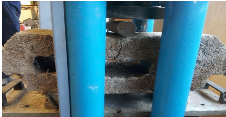
Figure B- 8: Flexural strength test hollow blocks
