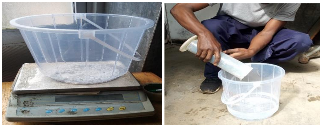
Figure B- 11: Weight of NaOH pellets per percentage and measurement of water
