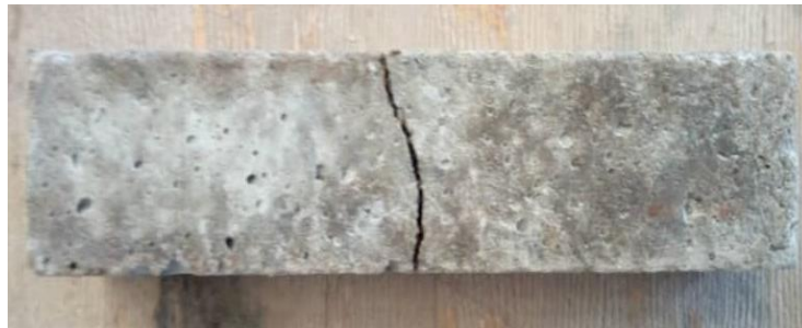
Figure B-4: Specimen with 0% BAMF after flexural test
