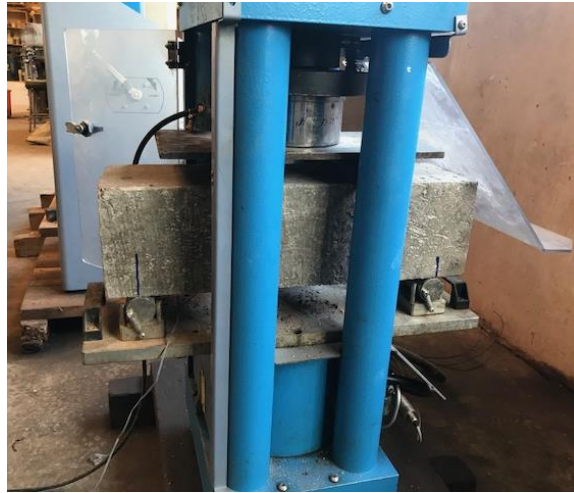
Figure 3-11: Set up of four points bending test on UTM.
