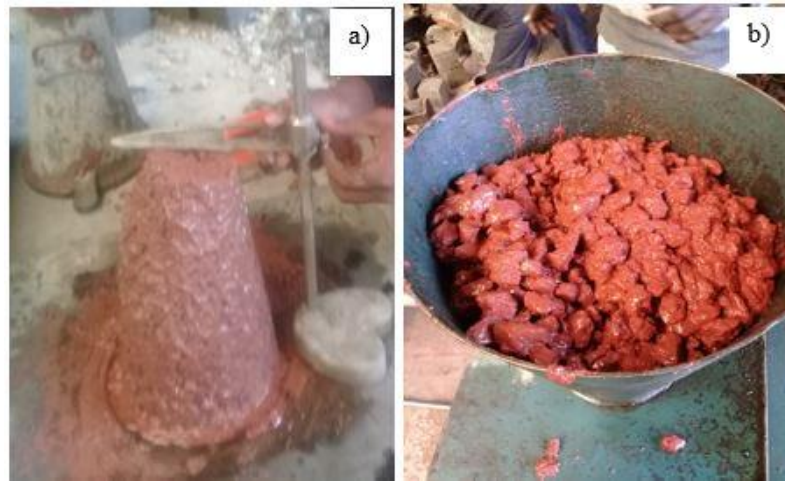
Figure 3-4: Slump measurement (a) and compaction factor test (b).
