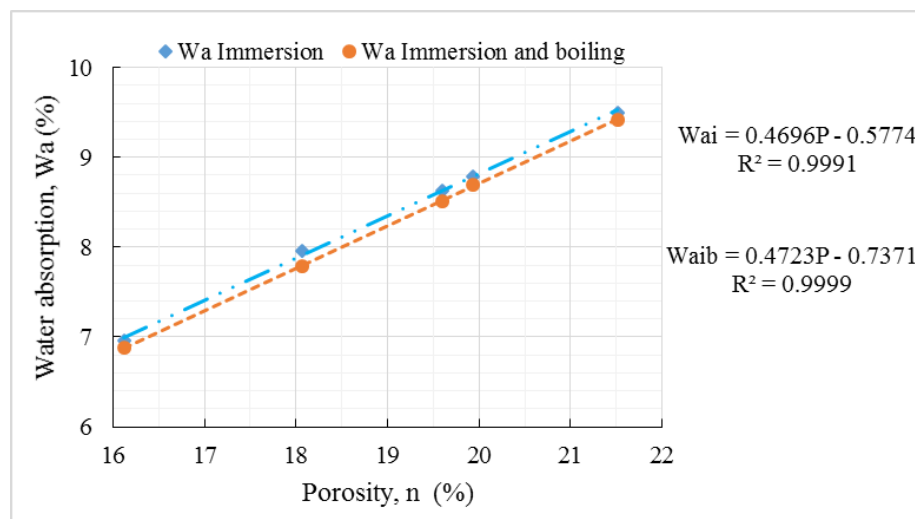
Figure 4-15: Relationship between water absorption and porosity.
