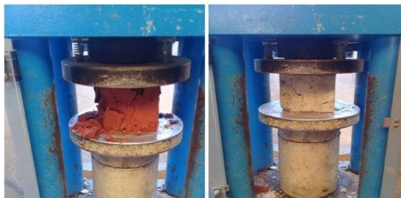
Figure 3-5: Compressive strength test.
