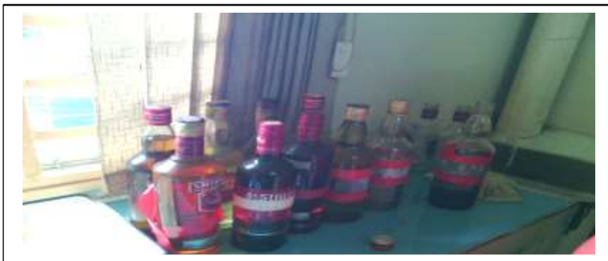
Figure 3.7: Samples of transformer oil in a well labelled and tightly sealed glass containers
