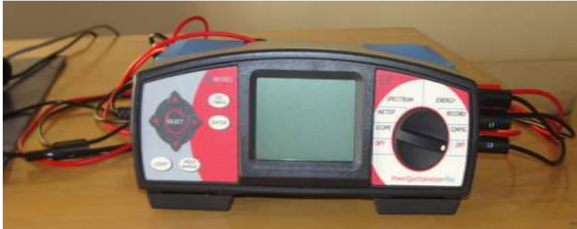
Figure 3.5: PQA employed in measurement of current harmonics at LV side of sampled distribution transformers
