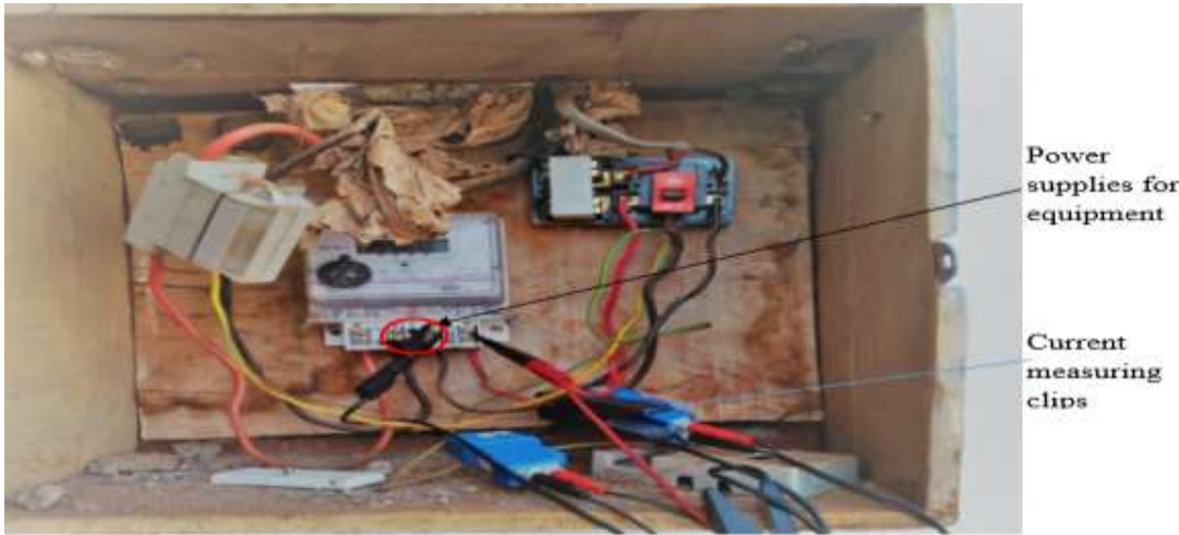
Figure 3.2: Connection of measuring equipment at point of common coupling (PCC)
