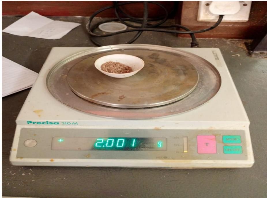
Figure 4: Precisa 310M analytical balance measuring briquette sample in a crucible
