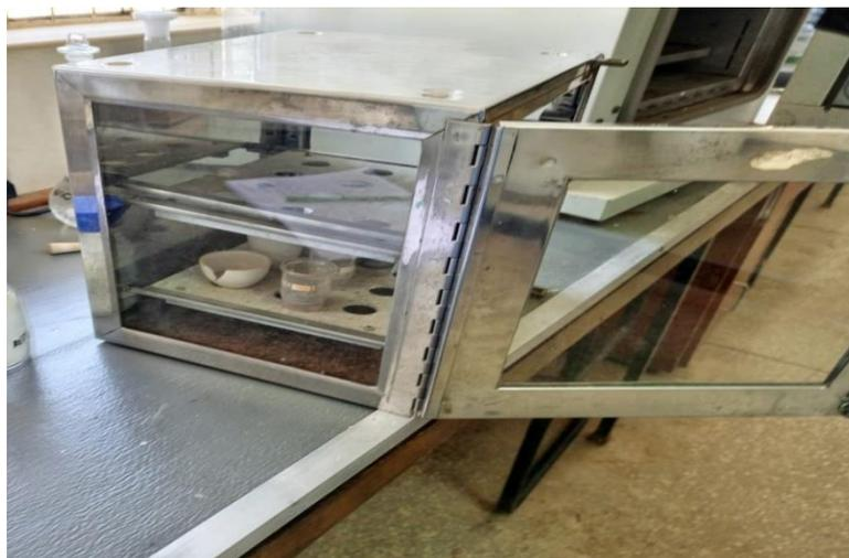
Figure 5: Desiccator containing desiccant
