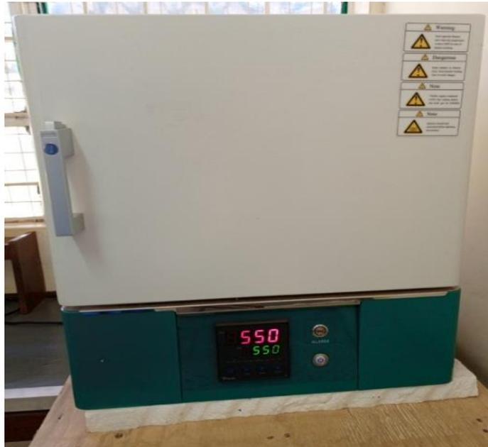
Figure 0: Ceramic fibre Faithful Model SGS Muffle furnace
