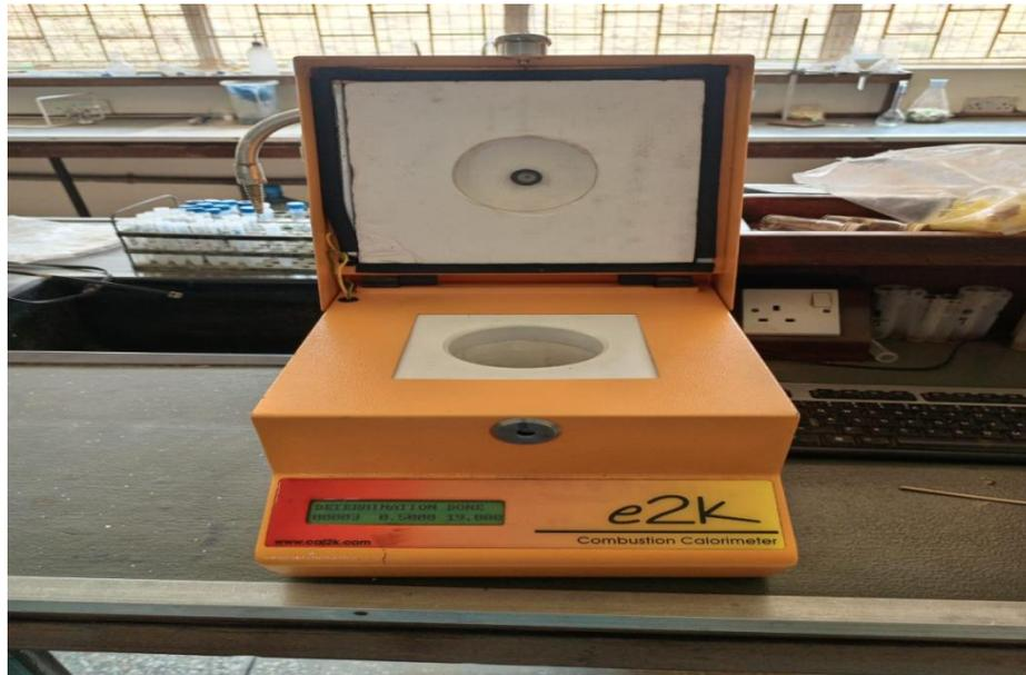
*Figure 6: e2K Combustion Calorimeter*
