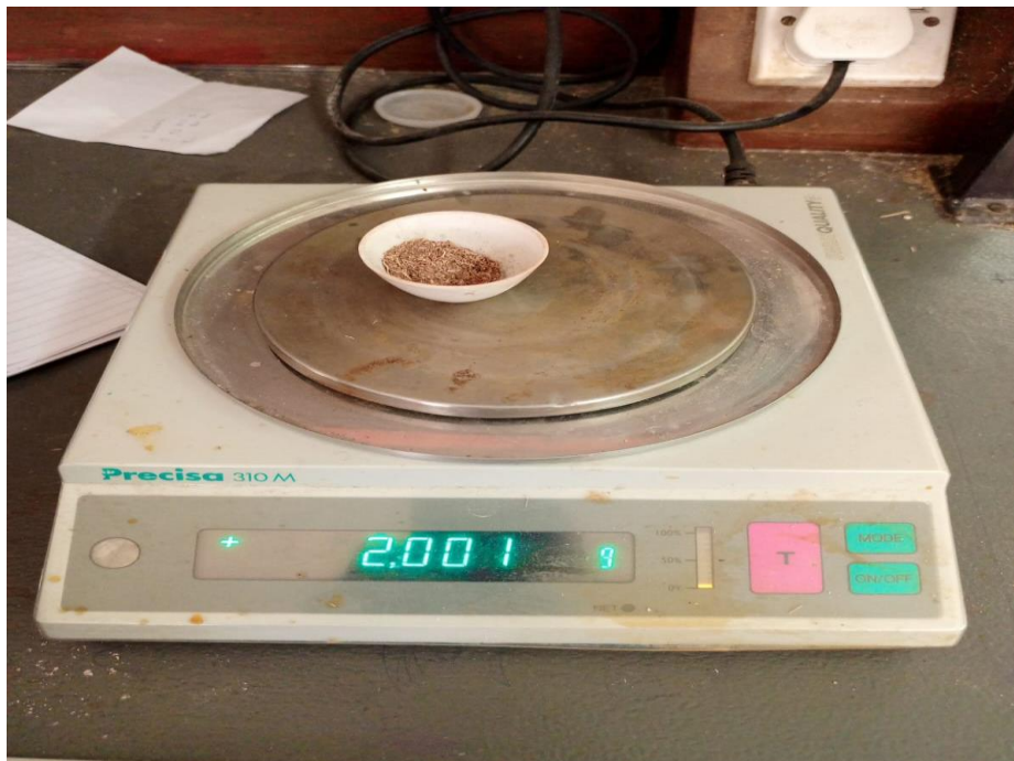
Figure 3.7: Precisa 310M by Precisa Gravimetrics AG-Switzerland, Analytical Balance Measuring Briquette Sample in A Crucible
