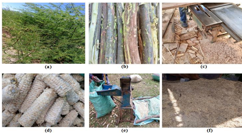
Figure 3.3: Feedstock Used; (a) Prosopis juliflora Tree,(b) Prosopis Logs, (c) Prosopis Logs being Grinded, (d)Maize Cobs,(e)Maize Cobs being Grinded and (f) Bagasse Feedstock
