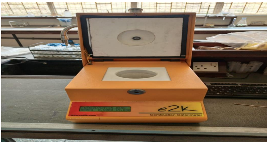
Figure 3 9: e2K Combustion Calorimeter by Digital Data Systems (Pty) Ltd – South Africa
