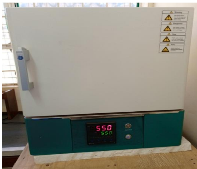
Figure 3.6: Ceramic Fibre Faithful Model SGS Muffle Furnace Manufacture by FAITHFUL Instrument Co. Ltd-China
