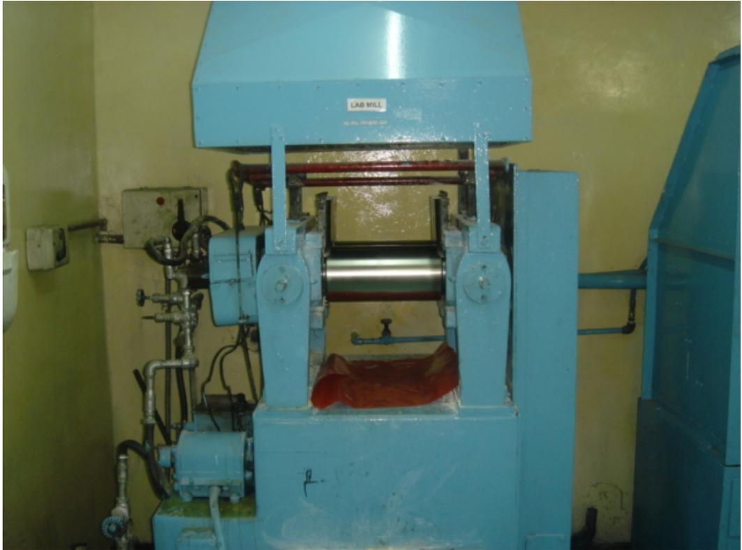
**Figure 3.1: Laboratory mill**
