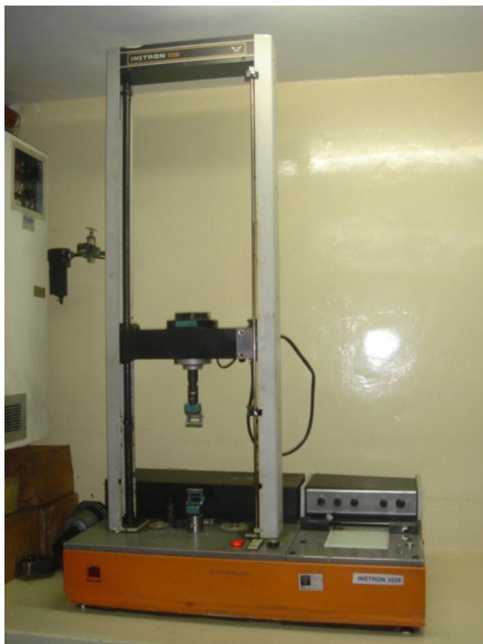
**Figure 3.4: Instron 1026 tensometer**
