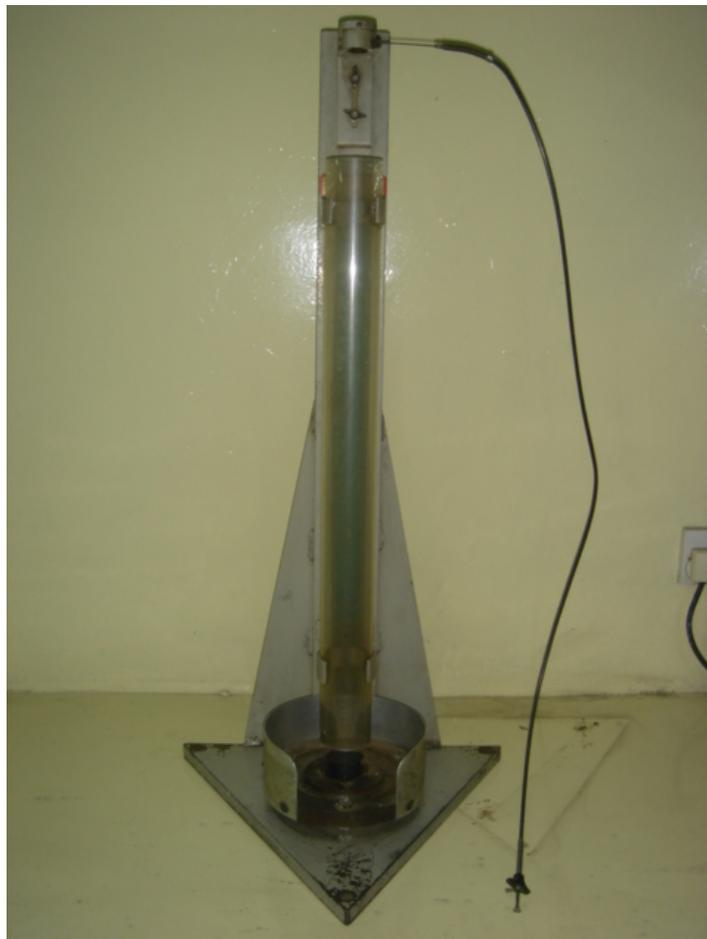
**Figure 3.5: Akron vertical rebound apparatus**
