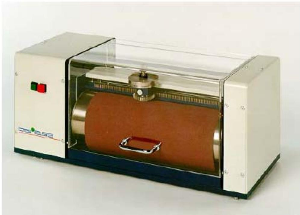
**Figure 3.6: DIN abrader apparatus**
